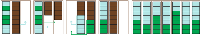
Fig. 6. The left four figures illustrate the process of sorting a single stack into two contiguous blocks. The last figure is the end result of applying the procedure to all stacks.
