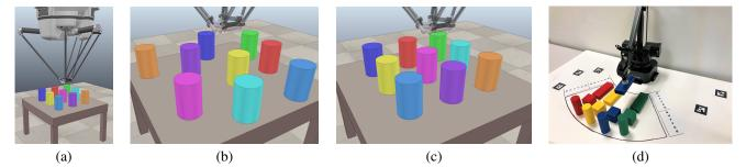
Fig. 2. (a, b, c) An example of an object rearrangement challenge considered in this work from a V-REP simulation [4], where the initial (b) and final (c) object poses are overlapping and an object needs to be placed at an intermediate location. (d) In addition to the V-REP simulations, the solutions presented in this work have been tested on an experimental hardware platform.
