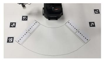
Fig. 17. A tabletop environment where the uArm Swift Pro's workspace is the area between  $[45^\circ, 135^\circ]$  at a distance ranging between 140mm and 280mm from the base.
