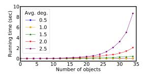
Fig. 12. The running time of ILP-Constraint under varying  $G_{dep}$  average degree. Maximum degree is capped at twice the average degree.
