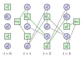
Fig. 23. An example of ILP model when n = 2, p = 1 as well as value of variables after solving this model. The green square nodes and green solid edges indicate the value of variables is 1. The solution is interpreted as (i) bring  $o_1$  to a buffer, (ii) bring  $o_2$  to its goal, (iii) bring  $o_1$  to its goal.
