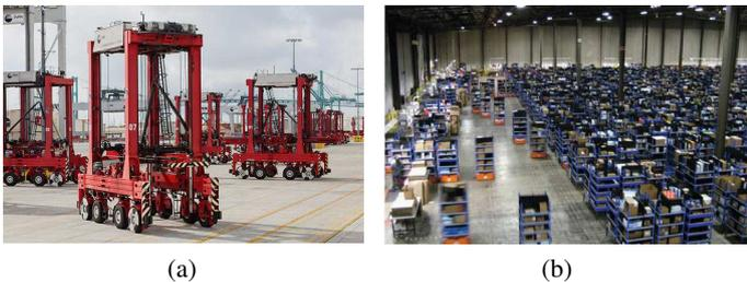
Fig. 1. (a) Automated straddle carriers at the port of Los Angeles. Each straddle carrier is capable of autonomously navigate to pick up or drop off a shipping container at a designated location. (b) Amazon’s Kiva multi-robot system working at its order fulfillment centers.
