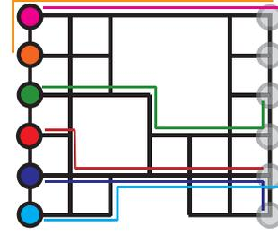
Fig. 1. A  $6 \times 7$  grid with some vertices removed. The colored discs on the left represent the initial formation and the gray discs the goal formation. The colored paths represent the paths (not yet scheduled to avoid collision).
