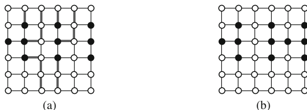
Fig. 1 Examples of the escape problem on a 6 \times 6 grid. The black discs are the initial evader locations. The goal is to plan disjoint paths for the evaders to reach different vertices on the boundary of the grid. a) An instance with solution given as the bold edges. b) An instance without a solution.
